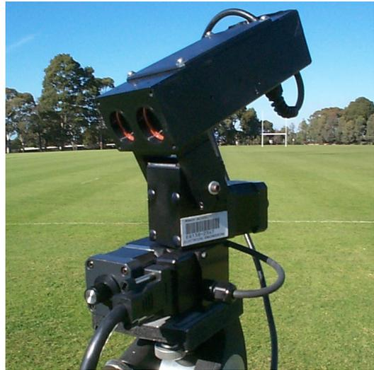
Figure 1: Laser Sensor and Pan-Tilt Unit
